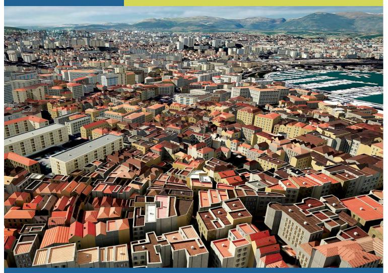
LuxCarta is building on its BrighEarth™ technology to add "smart" textures derived by artificial intelligence (AI) to its building polygons. Information on roof type and color, as well as facades, is synthesized using AI from the imagery to provide realistic textures cost effectively.
